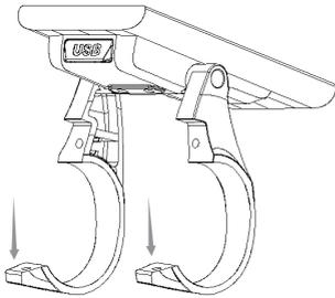
2. Now place the display on to the handlebar in the correct position. Now with 2 X M3\*12 screws tighten the display into position. Torque requirement: 1N.m.
