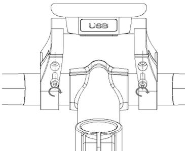
3. Open the clamp on the D-pad and place it in the correct position, Using 1 X M3\*10 screw tighten the D-pad onto the handlebar. Torque requirement: 1N.m.
